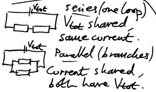
Resistor converts electrical E into thermal, due to its Resistance (Symbol: R) (Unit:  $\Omega$ )
